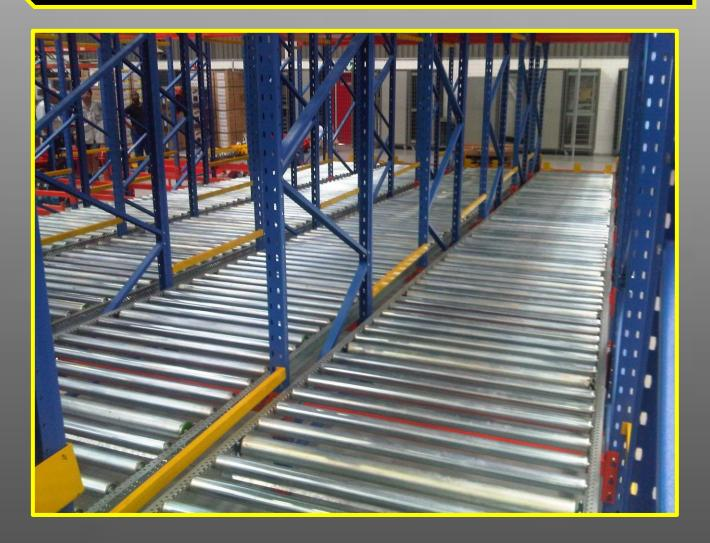
Acrow provides the Pallet Flow Systems and their supporting rack which in turn ensure a First in First out operation. This allows for the greatest pallet density possible and only a loading face and offloading face, thus keeping aisles to a minimum and forklifts out of the racking. A push-back system can also be accommodated.
